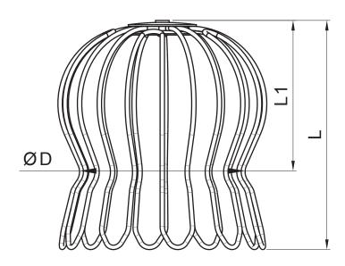
The dimension D is changed by pushing into the hole in the gutter (rain-water hopper)
