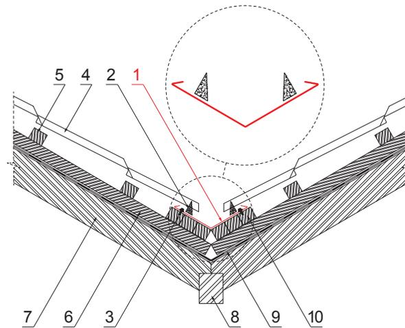
A sealing strip is glued to the fixed roof valley. It is covered with roof covering. The position of the sealing strip should be such that it is not affected by sunlight (it must be sufficiently covered by roof covering). The strip prevents water from entering under the covering.
