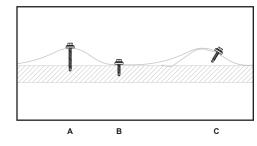
Correct setting of the tightening torque when anchoring the screws:
