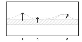
Correct setting of the tightening torque when anchoring the screws:
