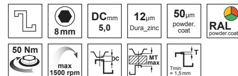
Correct setting of the tightening torque when anchoring the screws:
