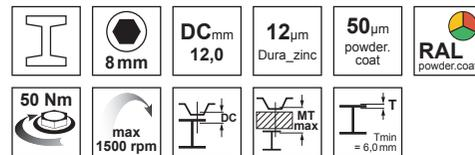
Correct setting of the tightening torque when anchoring the screws:
