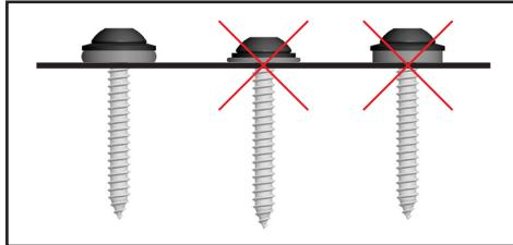
Correct setting of the tightening torque when anchoring the screws:
