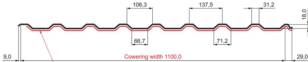
SQ = ANTI-CONDENSING AND ANTI-NOISE FELT th. 3–4 mm
