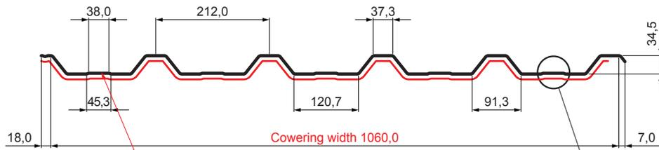
SQ = ANTI-CONDENSING AND ANTI-NOISE FELT th. 3–4 mm
