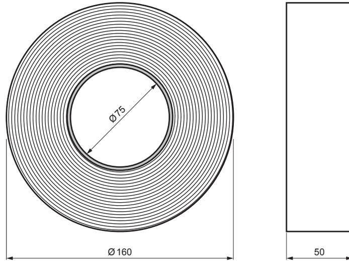
Single-sided tape made of polypropylene non-woven and acrylic dispersion adhesive. Designed for sealing and repairing roof membranes and other construction materials based on polypropylene. The tape protects against the penetration of moisture and wind while maintaining the vapour permeability of the membrane, whose surface breathes.
