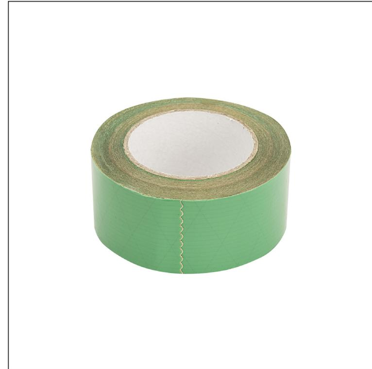
Universal single-sided PE tape reinforced with polyester fibre and special adhesive based on acrylic dispersion. It is generally used in the construction industry, especially for bonding and repairing foils and roof membranes made of plastic and their bonding with wooden and metal elements. It is also used for bonding other construction products based on plastics.
