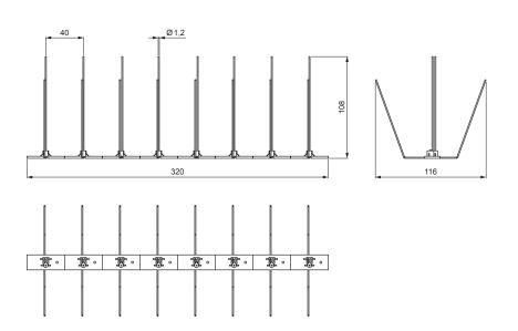
The universal spike system H113 is suitable for repressive treatment of surfaces up to 180 mm in width, or cylindrical surfaces of 120 mm in diameter. The spikes protect the surface and the space above the surface. They will prevent pigeons from perching on the surface and thereby they will also prevent pollution. The spikes can be used for treatment of structural elements up to a width of 80 mm.
