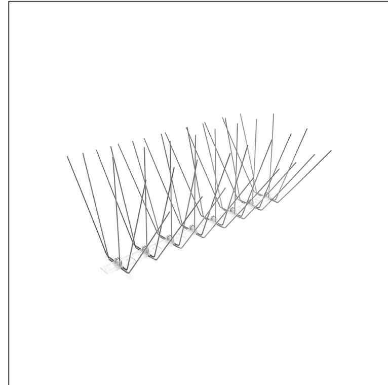
The universal, highly efficient H126 spike system is suitable for repressive treatment of cornices up to 250 mm or structural elements up to 170 mm in width. High efficiency is ensured by an extremely large number of spikes (125 pcs). per standard meter and its construction is one of the densest systems of this design in Europe.
