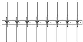
The universal, highly efficient H126 spike system is suitable for repressive treatment of cornices up to 250 mm or structural elements up to 170 mm in width. High efficiency is ensured by an extremely large number of spikes (125 pcs). per standard meter and its construction is one of the densest systems of this design in Europe.
