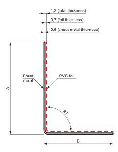
SHEET METAL WITH PVC is a double-sided hot-dip galvanized sheet with a laminated PVC foil in colour on the front side and with a cover varnish on the reverse side. The laminated sheet is manufactured according to STN EN 10169+A1 a STN EN 14783.
