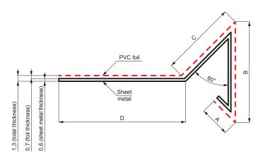
**SHEET METAL WITH PVC** is a double-sided hot-dip galvanized sheet 275 g/m² with a laminated PVC foil in colour on the front side and with a cover varnish on the reverse side. The laminated sheet is manufactured according to STN EN 1849-1, STN EN 1297 and STN EN 4102.
