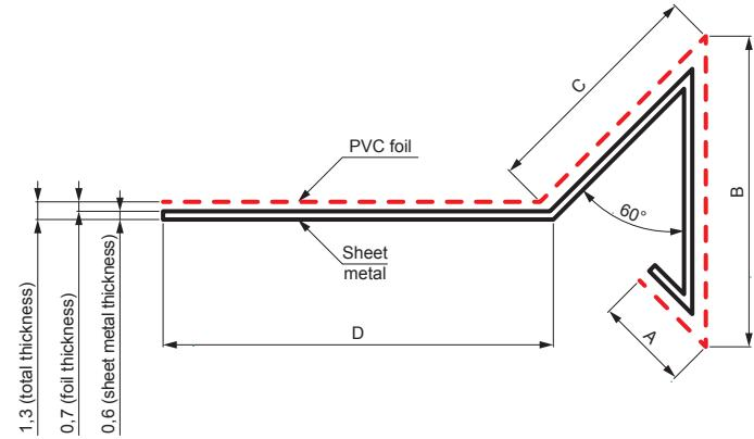
**SHEET METAL WITH PVC** is a double-sided hot-dip galvanized sheet 275 g/m<sup>2</sup> with a laminated PVC foil in colour on the front side and with a cover varnish on the reverse side. The laminated sheet is manufactured according to STN EN 1849-1, STN EN 1297 and STN EN 4102.
