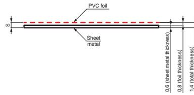
**SHEET METAL WITH PVC** is a double-sided hot-dip galvanized sheet with a laminated PVC foil in colour on the front side and with a cover varnish on the reverse side.
