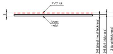
**SHEET METAL WITH PVC** is a double-sided hot-dip galvanized sheet with a laminated PVC foil in colour on the front side and with a cover varnish on the reverse side.
