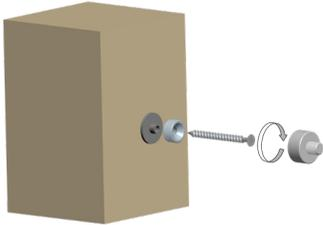
**1** rubber pad, bottom part, wood screw, platform top part
