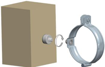
**3** screw the upper part onto the bottom part and screw the sleeve on
