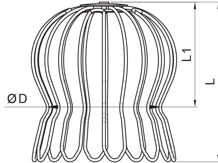
The dimension D is changed by pushing into the hole in the gutter (rain-water hopper)
