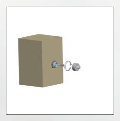
fasten the platform bottom part with a pad using the wood screw
